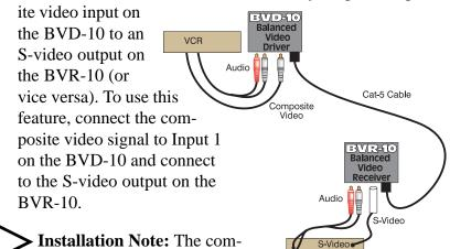
> Installation Note: The composite to S-Video feature does not function on Video Input #2.
