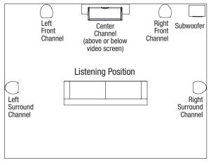
Figure 1: This overhead view shows a typical wall mounted 5-channel home theater plan.
