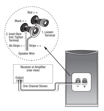
Figure 8: Wiring diagram shows polarity connections for one channel of an audio system.
